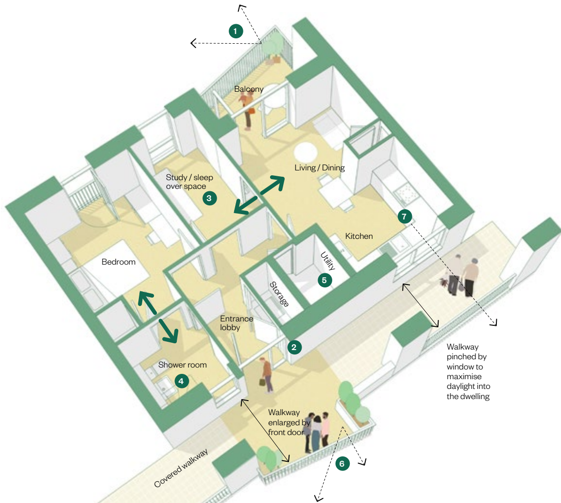
Fig 125 Example of older people's apartment following HAPPI principles (Carlton Dene Extra Care by Levitt Bernstein)
