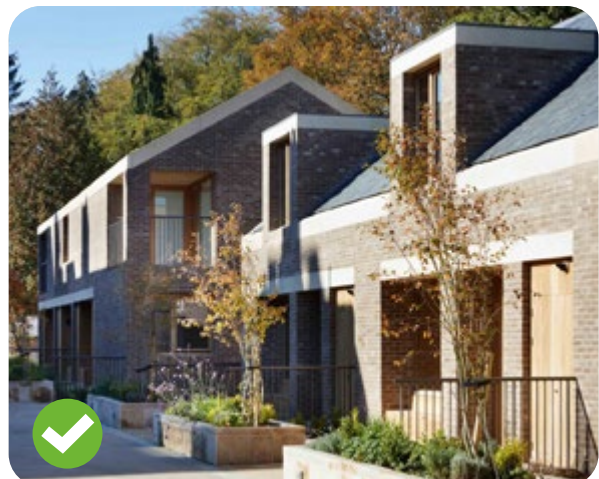
Fig 108 Small set backs along the building line are opportunities to introduce trees and soft landscaping (Wilderness Mews by Morris + Company)
